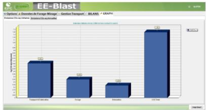
**The energy consumption** will depend on the resulting grain size obtained after blasting. This tool allows the optimization the chain by choosing the appropriate fragmentation energy level, which reduces the energy consumption of the whole operation. We were able to demonstrate that energy optimization and reduction of the carbon footprint are associated with productivity.
